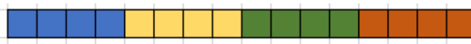
1D representation of tiles showing how it can be treated as a 2D representation by joining each row
